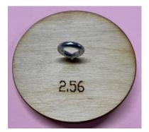
1) Apply some glue to the hole in the bulkhead and screw the screw eye into the bulkhead.
