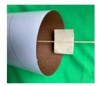
7) When the parachute ejects at apogee, the main body tube can be damaged by the thin Kevlar shock cord mount. The Kevlar cord can cut into the top of the body tube and tear a thin opening down the tube. This is called a zipper. The chance of zippering can be lessened by wrapping some masking tape around the Kevlar cord at a location that extends just above and below the top of the body tube.
