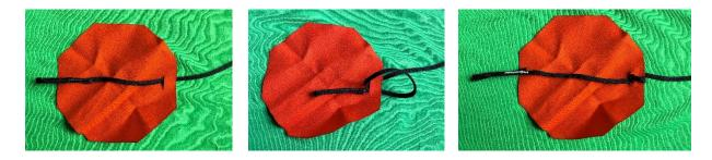
3) Use a *follow-through figure eight loop knot* to attach the Kevlar shock cord mount to the loop in the free end of the nylon shock cord. See <u>www.animatedknots.com/figure-8-follow-through-loop-knot</u> for an animation of the knot. Secure the loose Kevlar end with several half hitches.
