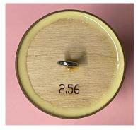
7) Apply a fillet of glue between the bottom of the bulkhead and the coupler. Allow glue to set.
