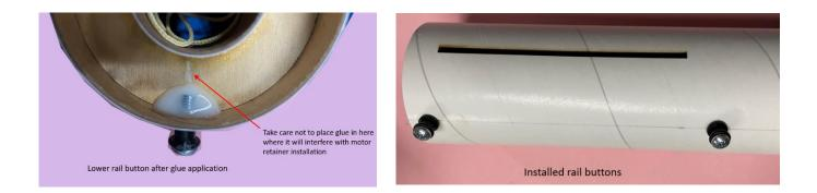
When gluing the upper rail button screw, you will need to reach down from the top with a long stick to place the glue. Be sure to pull the Kevlar shock cord mount down through the motor tube to avoid getting glue on the Kevlar cord.
