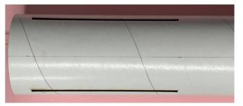
1) Measure halfway between two fin slots and place a mark on the body tube. Draw a 10-inch line through the mark starting at the bottom of the body tube.
