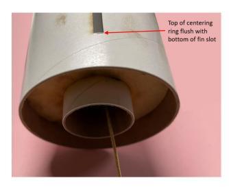
5) Slide the motor tube assembly into the bottom of the main tube until it hits the glued area. Continue pushing the tube in until the top of the lower centering ring is flush with the bottom of the fin slots. Check all three fin slots to be sure the centering ring is not blocking any part of any fin slot opening. If so, move the motor tube assembly downward so no fin slot is blocked.
