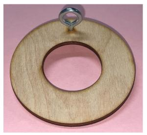
3) Screw one screw eye into the upper centering ring.
