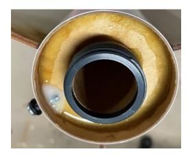
4) Press the motor retainer ring over the motor mount tube until it seats firmly on the motor tube. Wipe away any excess glue. Be careful not to get any glue on the retainer threads or inside the motor tube. If you do, wipe it off immediately before it sets.
