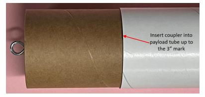
6) Insert the coupler into the end of the tube up to the half-way mark on the coupler. Make sure you do this quickly because the glue will set almost immediately! Position the assembly upright and allow the glue to dry.
