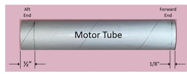
4) Mark the motor tube 1/8 inch from the forward end and  $\frac{1}{2}$  inch from the aft end.
