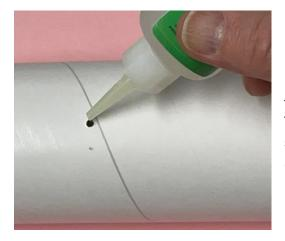
13) To avoid creating turbulence that may affect the altimeter reading, the pressure equalization holes should be smooth and square-edged. The hole left in the cardboard tube wall by the drill bit will be rough. To smooth the hole, start by placing a drop of thin CA glue in each hole and allow to dry. The rough cardboard edge will wick the CA glue and harden.
