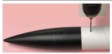
8) Mark a point 1 inch down from the top of the payload tube.
