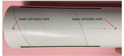
3) Measure from the aft end of the body tube to the bottom of the lower centering ring. Subtract 1/16 inch, and mark the resulting distance on the line drawn in step 1. Measure from the forward end of the body tube to the top of the upper centering ring. Subtract 1/16 inch, and mark the resulting distance on the line drawn in step 1.
