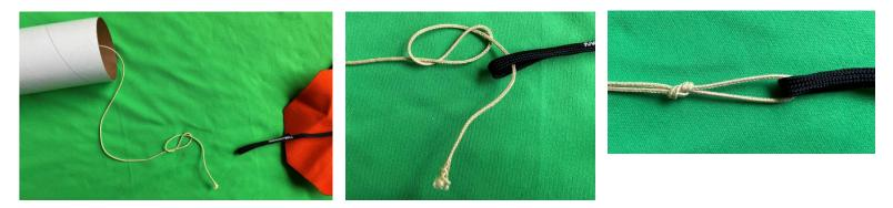
4) Measure 36 inches down from the nylon shock cord attachment point to the payload section (about 1/3 the length of the nylon shock cord) and tie an overhand loop knot. The loop should be about 1.5 inches long. This loop will be the parachute attachment point.
