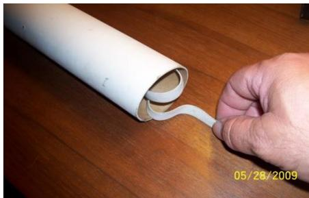
Feed in the remaining top portion of the shock cord, and then slide on the payload section of the rocket. **The two parts should go together snugly but *not* so tightly that excessive force is required to put the payload section in place.**
