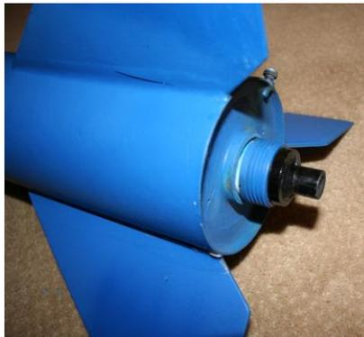
Slide the motor into the motor mount tube until the thrust ring on motor casing abuts the motor retainer.
