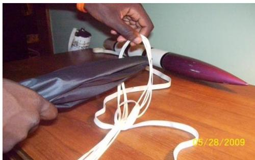
If your team followed the recommended assembly directions for the shock cord, there should be a 3 inch loop in the shock cord about two feet from the payload section. Feed the loops of the parachute shroud lines part way through the 3 inch loop of the shock cord. Take the top of the parachute and feed it through all the shroud line loops at once.
