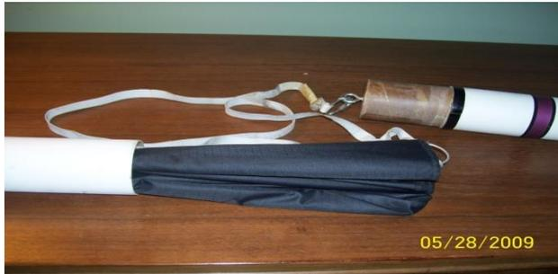
Insert the folded parachute with the shroud lines facing out the top of the tube. The parachute should not be packed in too tightly or it may not eject properly.
