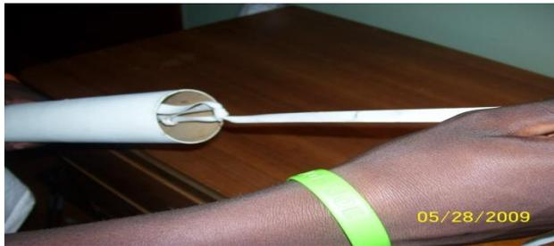
If the parachute is loaded correctly, it should slide out of the air frame with limited force. Test the packing of the chute by lightly pulling on the top part of shock cord to feel if the parachute starts to slide easily. If the packing seems too tight, pull out the parachute and refold it.
