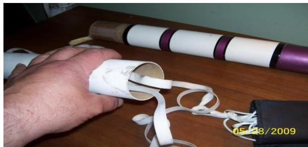
Feed the lower portion of the shock cord, below where parachute is attached, into the top of the air frame.
